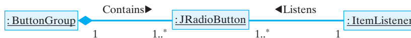
Figure 13.27: The ButtonGroup object tracks each radio button's state, ensuring that only one is selected at a time. The ItemListener listens for events on each button.
