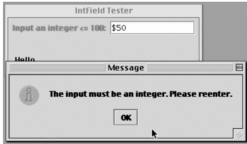
Figure 10.16: This exception handler opens a dialog box to display an error message.
